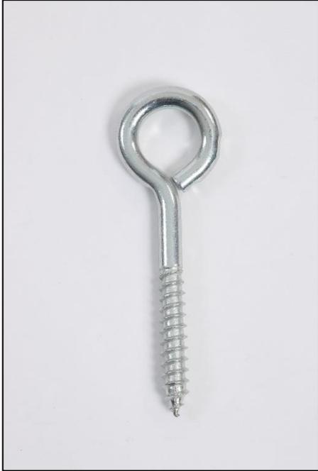
Locate the ceiling beam/joist by using a stud finder or tapping and verifying with a small nail. Be sure to locate the exact center of the ceiling joist for the most secure installation. Using a 3/16" (3mm) wood drill bit, drill a starter hole (approx. 4" or 10 cm deep) perpendicular to the ceiling. Screw in the supplied eye bolts until all threads have disappeared into the joist. Do not loosen or adjust once in place.
