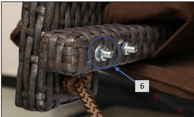
6. Insert a hex bolt (front to back) into each hole and tighten nut and washer using the wrench included in the kit. Tighten each bolt until it is flush with the front side of the wicker.
